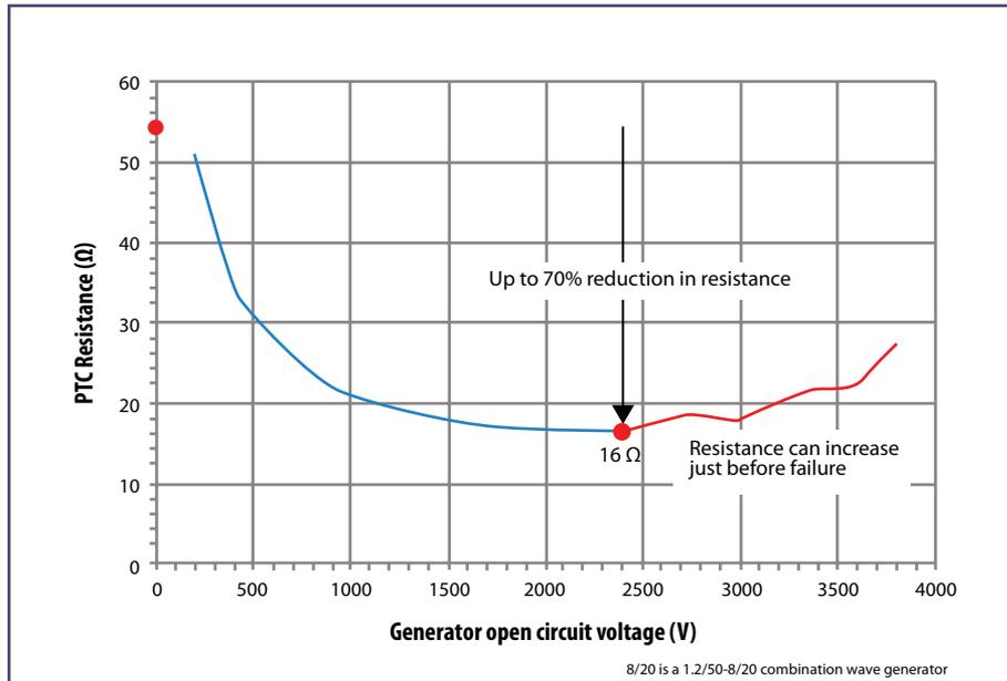
Figure 5. | CMF-RL55-0-A1 Resistance During 8/20  $\mu$ s
