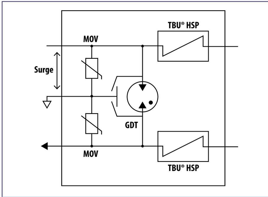
Figure 7. | Hybrid Primary and Secondary Protector
